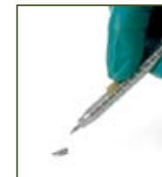
Step 6 Discard blade by advancing next screw
