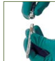
Step 2 Connect blade onto driver by pulling back on driver engagement and inserting end
